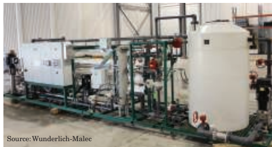
FIGURE 2. These complete, modular integrated water solutions are pre-assembled and factory tested to meet the client’s functional requirements
